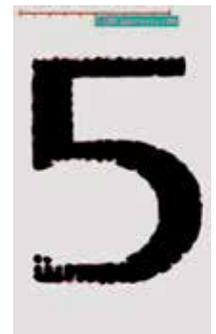
printed with standard high-modulus mesh
