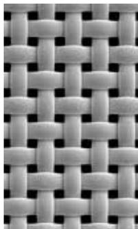
Mesh-opening with standard high-modulus mesh 150-34 PW (1:1)
